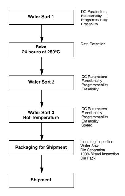
Figure 1. AMD KGD Product Test Flow
