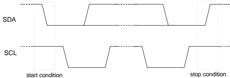
Start and stop conditions are generated by MCU. The buses are busy after a start condition is activated and are idle after a while when a stop condition is activated.
