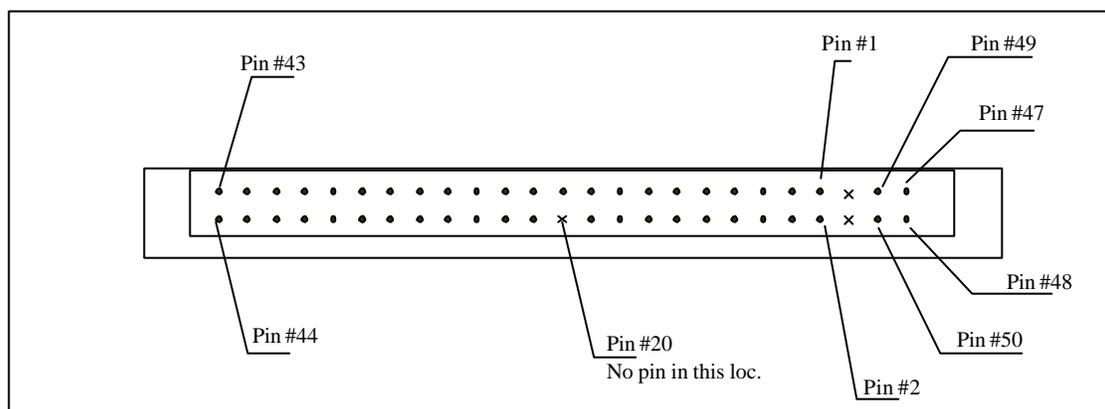
**Figure 2: Pin Configuration**
