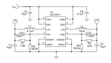
Figure 1: AAT2511 Adjustable Output with Enhanced Transient Response.
