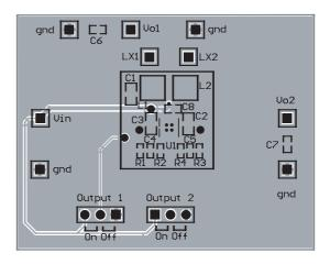
Figure 4: AAT2511 Evaluation Board Bottom Side.
