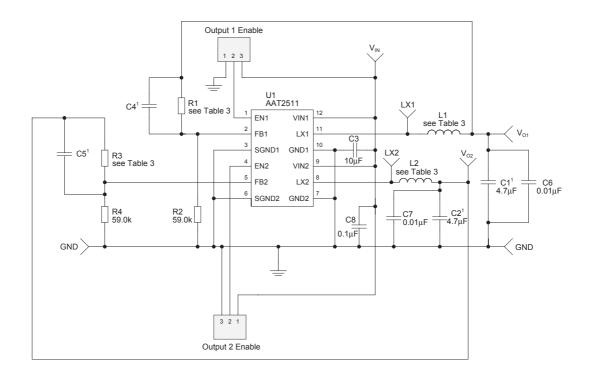
Figure 2: AAT2511 Evaluation Board Schematic.
