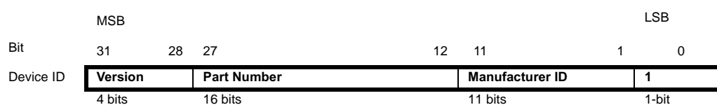
Figure 27-1. The Format of the Device Identification Register
