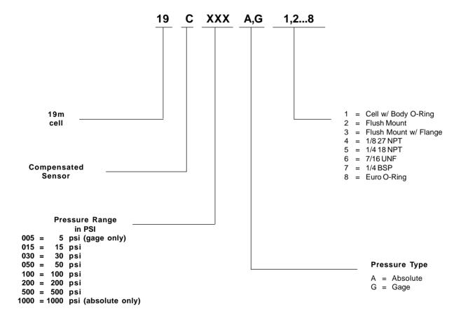
For example: Part #19C100A4 = 19 mm Cell, Compensated, 100 psi, Absolute, 1/8NPT Port
