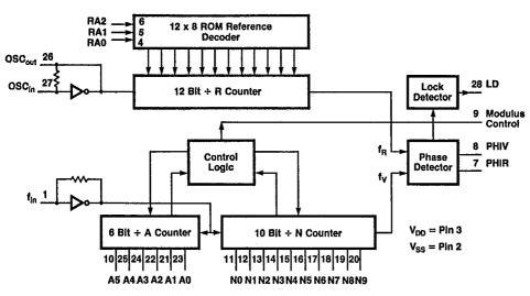
NOTE: N0 through N9, A0 through A5 and RA0 through RA2 have pullup resistors not shown.
