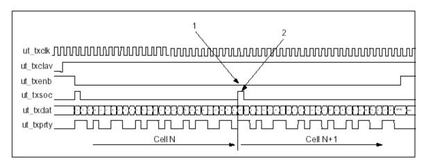
Figure 7: Back to Back Cell Transfer - Cell Level Transfer
