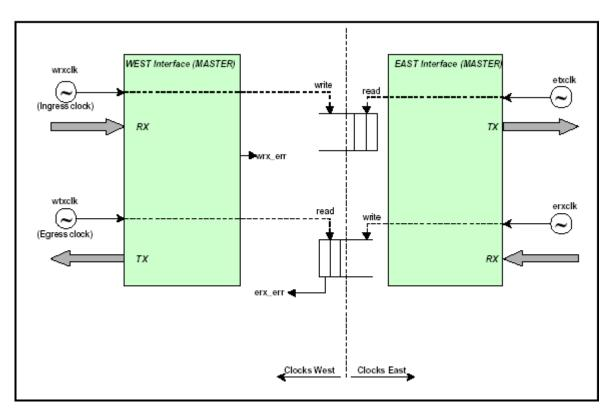
Figure 5: Master/Master Bridge Clock Distribution
