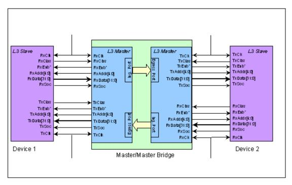
Figure 3: Master/Master Bridge connecting two Slave Devices
