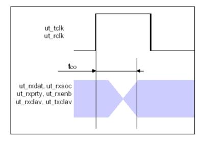
Figure 11: Tco Timing Parameter Definition
