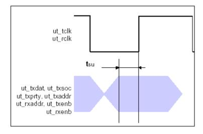
Figure 12: Tsu Timing Parameter Definition
