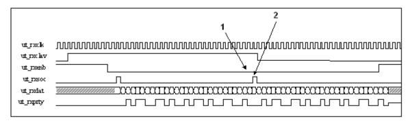
Figure 9: Back to Back Cells Transfer - Cell Level Transfer
