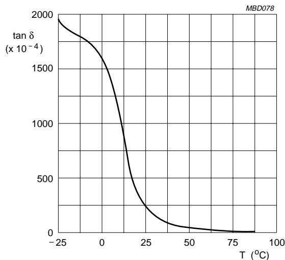
Fig.4 Typical  $\tan \delta$  as a function of temperature.
