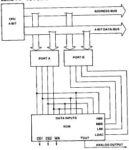
This figure shows how to operate the HS 9338 with two 4-Bit ports. The chip-selects are tied to ground allowing continuous operation; they can be used for operating more DAC's at the same port. In the first step data should appear at the port A outputs; in the second step the control flags should appear on port B.
