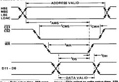
t<sub>DS</sub>: Data setup time, 250 neec t<sub>DH</sub>: Data hold time, 20 neec
