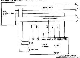
This mode of operation requires 13k bytes of unused addresses. No additional address decoder is necessary. The two chip-select input together with the byte-enable and load-DAC inputs are used to control all functions of the DAC. Through selecting the address-lines the user can vary the addresses used to control the DAC. In the above figure the control signals have the following address-configurations (hex):
