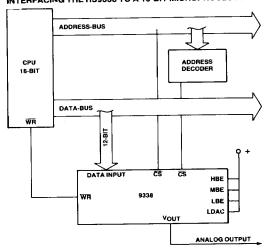
Interfacing the HS9338 to a 16-Bit microprocessor is quite easy, because no multiplexing of the data inputs is necessary. An address decoder and the second chip-select input is used to select the DAC.
