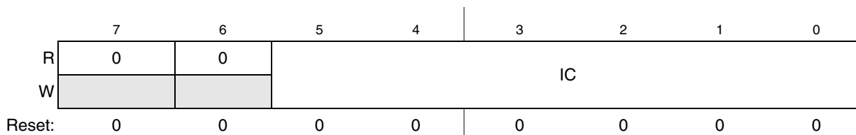
Figure 22-10. I 2 C Frequency Divider Register (I2FDR)
