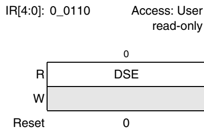
Figure 27-3. 1-Bit TEST_CTRL Register
