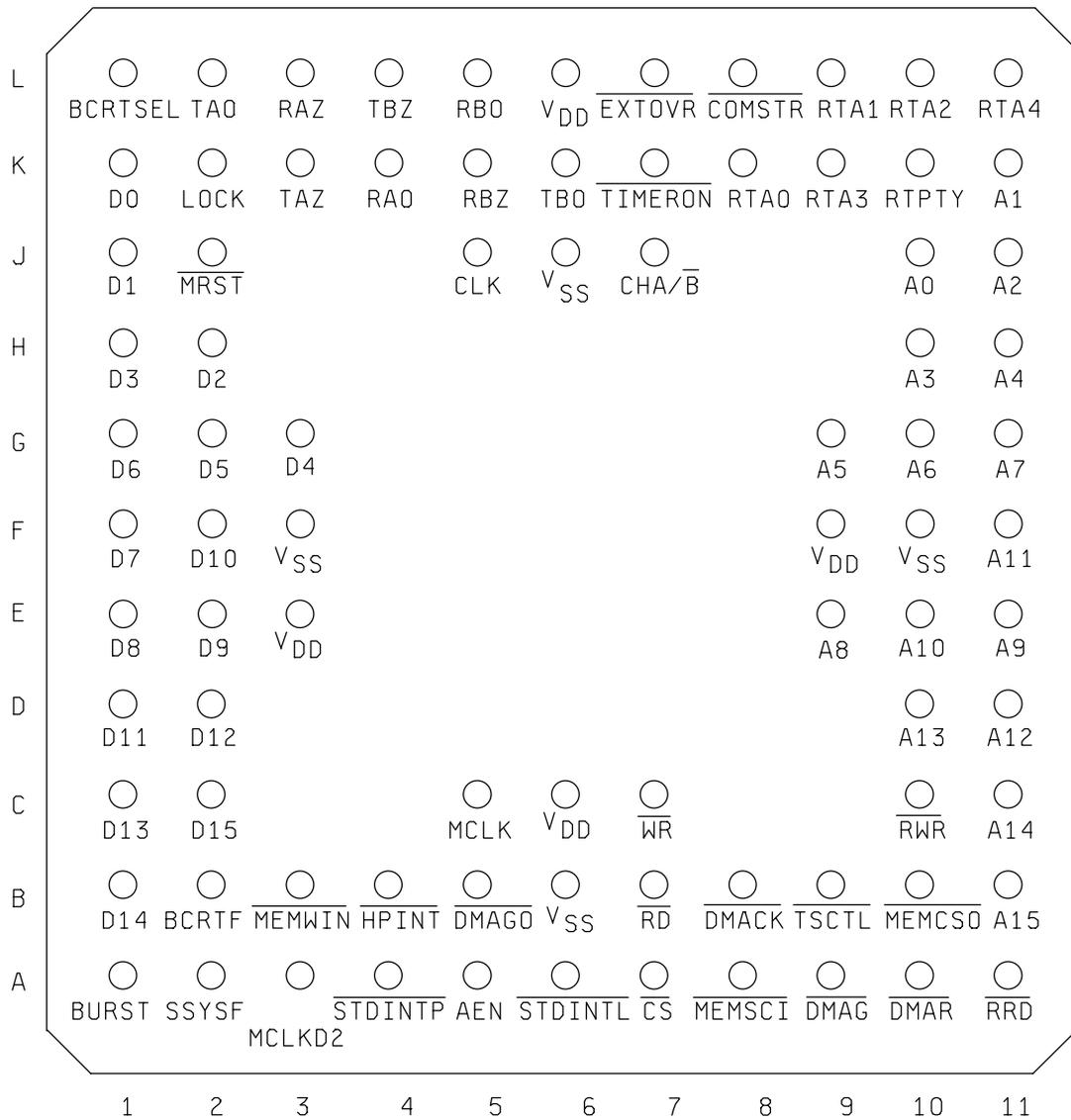
NOTE: MEMWIN is an internal test pin only and should be considered a floating pin and not for use.
