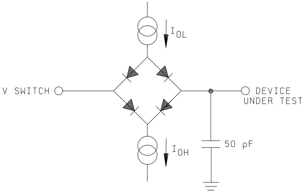
FIGURE 3. Switching test circuit and waveforms.
