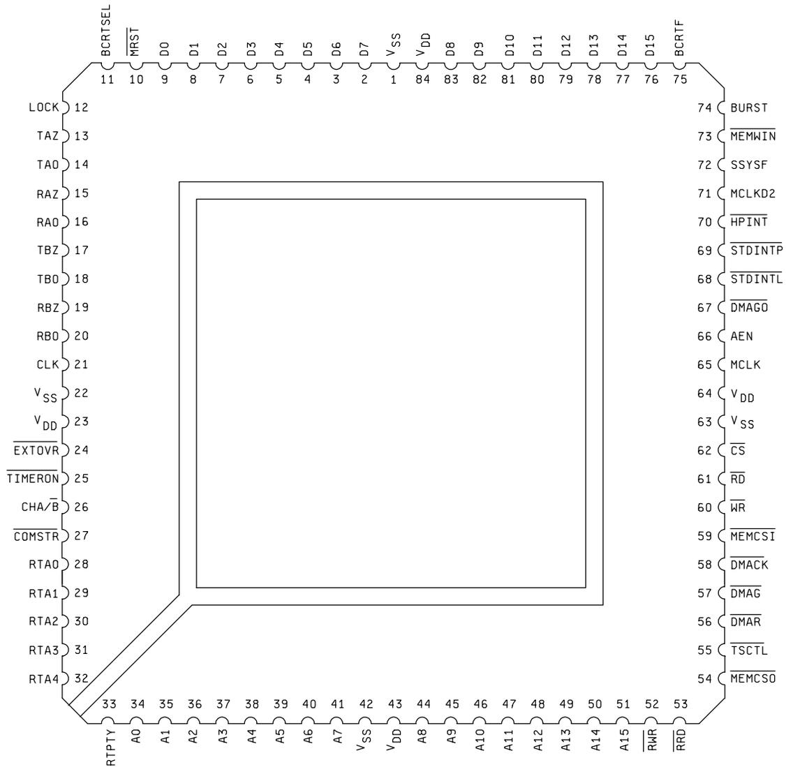
NOTE: MEMWIN is an internal test pin only and should be considered a floating pin and not for use.
