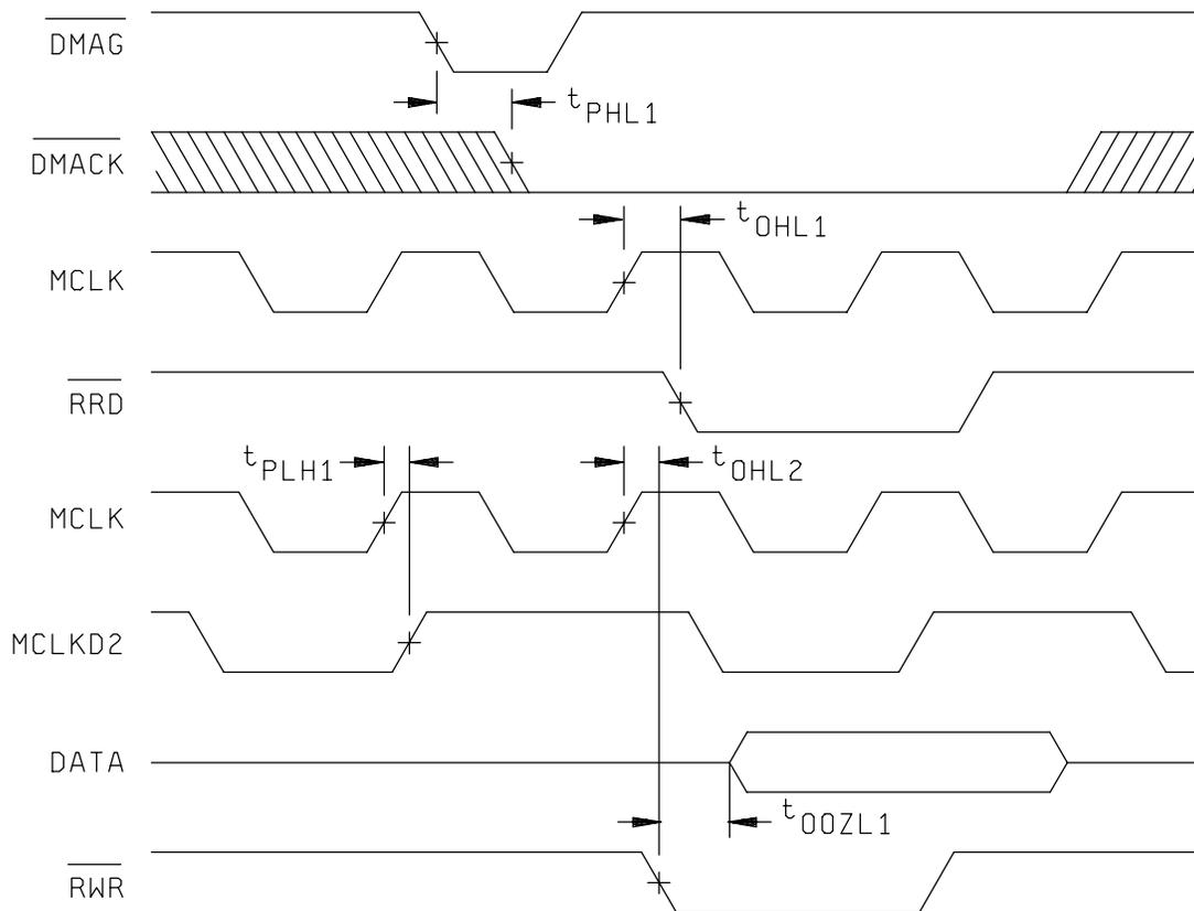
FIGURE 3. Switching test circuit and waveforms. - Continued
