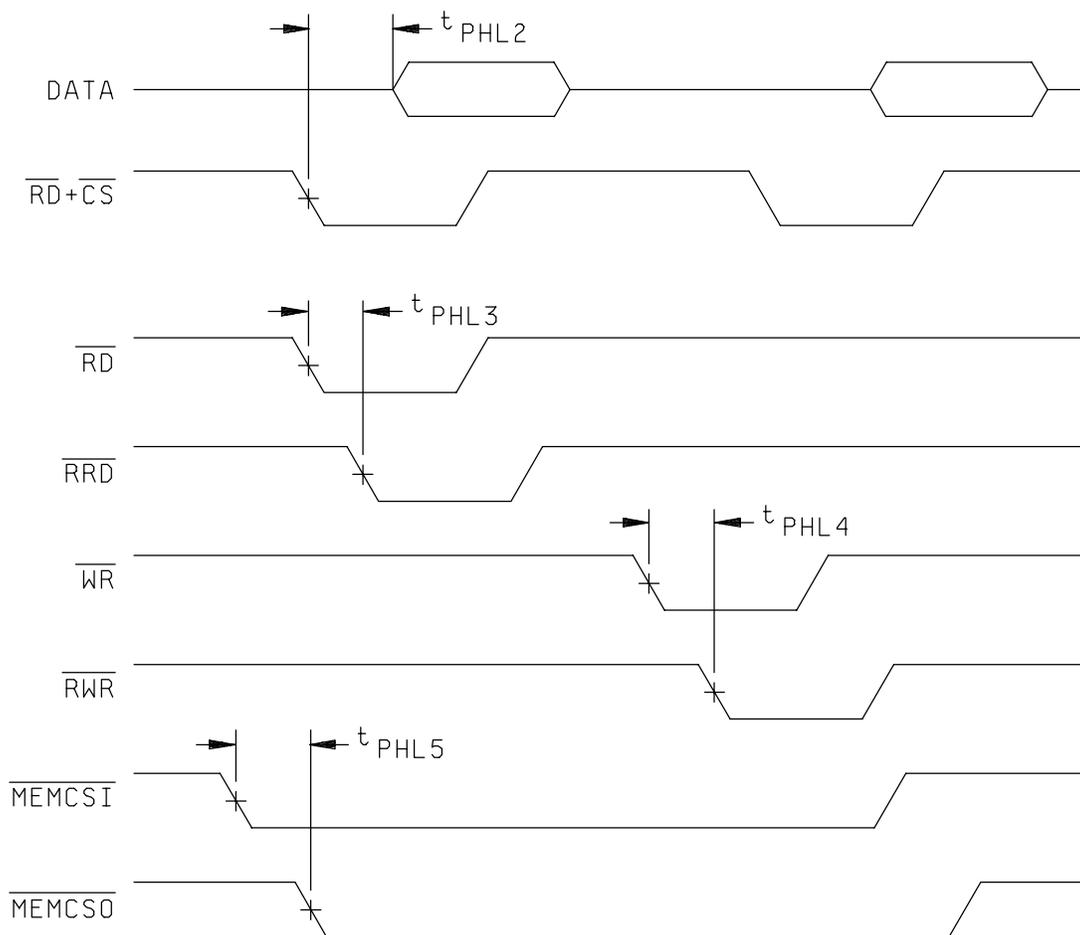
FIGURE 3. Switching test circuit and waveforms. - Continued
