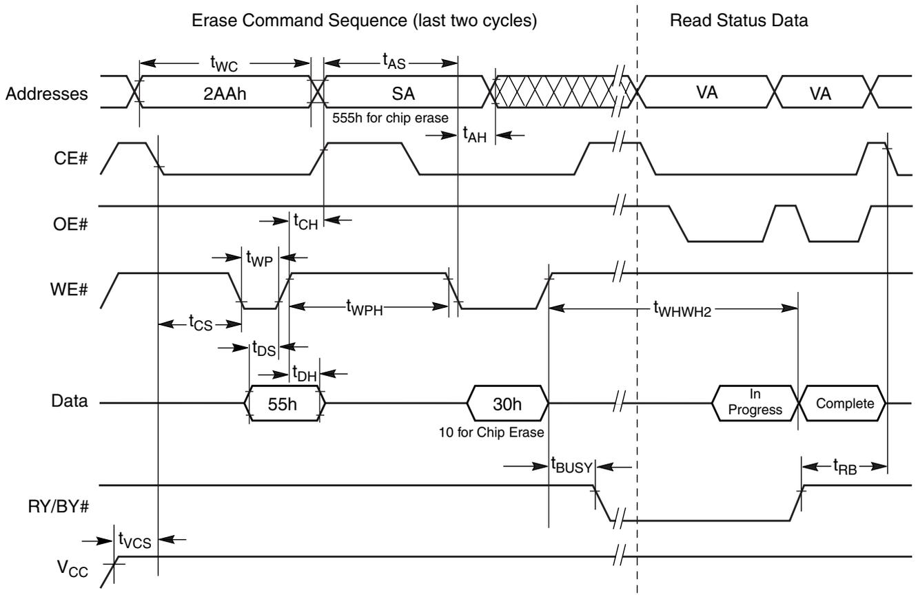
**Note:** SA = sector address (for Sector Erase), VA = Valid Address for reading status data (see "Write Operation Status").
