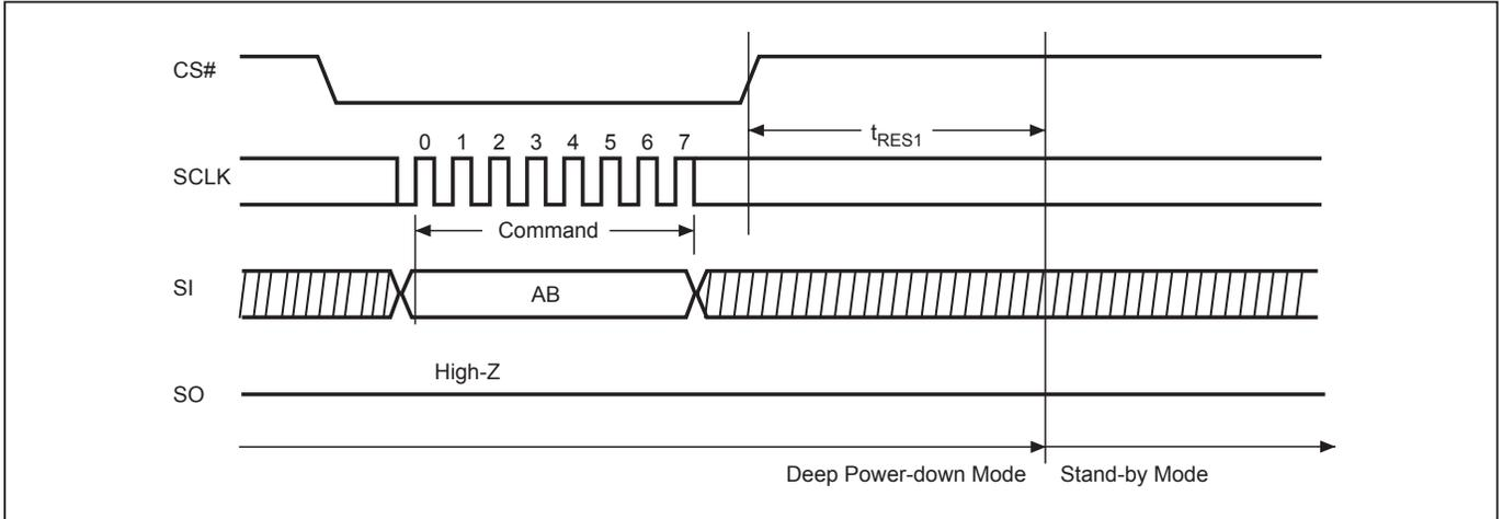
**Figure 30. Read Electronic Manufacturer & Device ID (REMS) Sequence (Command 90 or EF or DF)**
