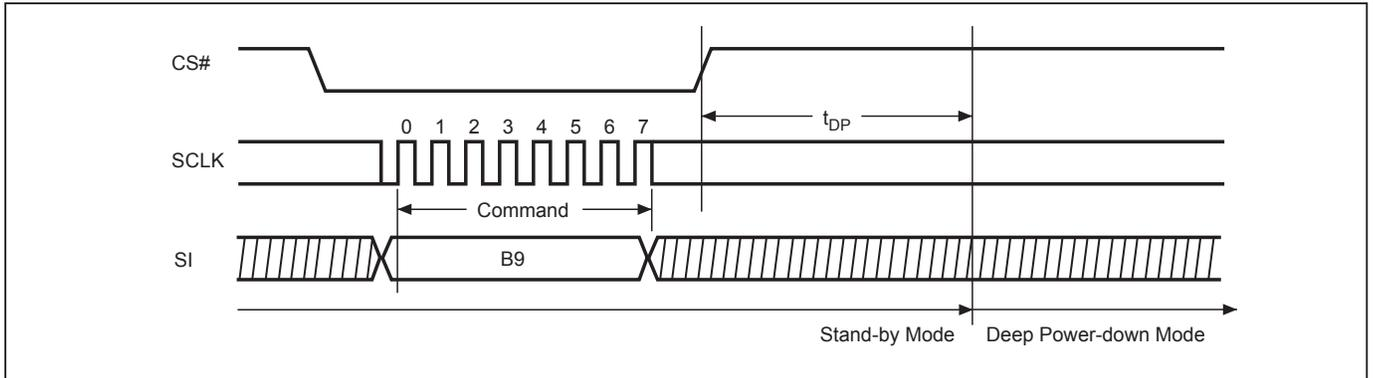
**Figure 28. Release from Deep Power-down and Read Electronic Signature (RES) Sequence (Command AB)**
