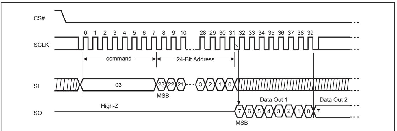
Figure 16. Read at Higher Speed (FAST\_READ) Sequence (Command 0B)
