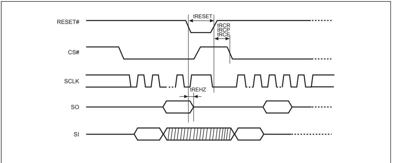
**Figure 10. Write Enable (WREN) Sequence (Command 06)**
