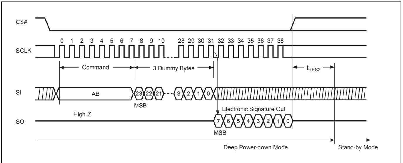
**Figure 29. Release from Deep Power-down (RDP) Sequence (Command AB)**
