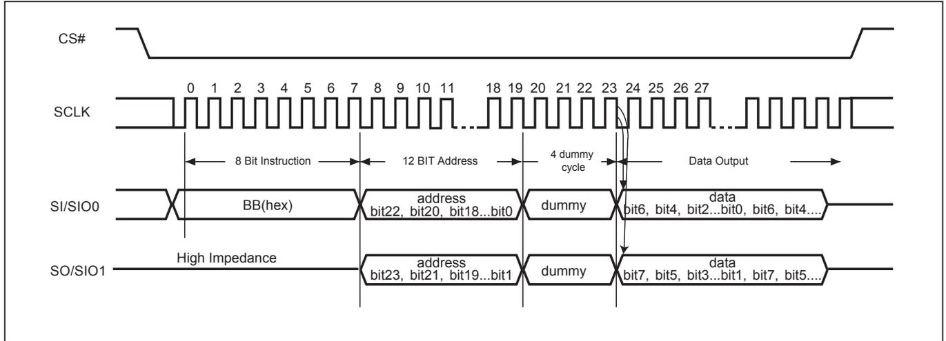
**Figure 18. 4 x I/O Read Mode Sequence (Command EB)**
