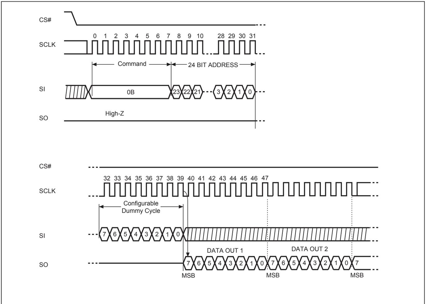
**Figure 17. 2 x I/O Read Mode Sequence (Command BB)**
