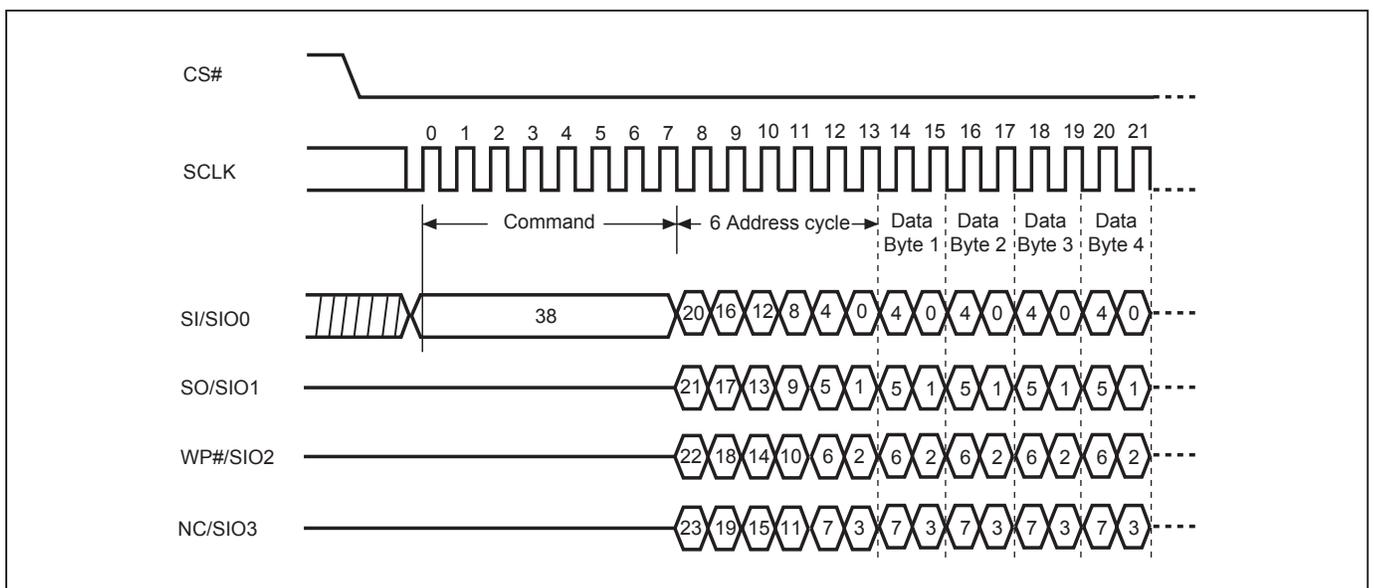
**Figure 22. Continously Program (CP) Mode Sequence with Hardware Detection (Command AD)**
