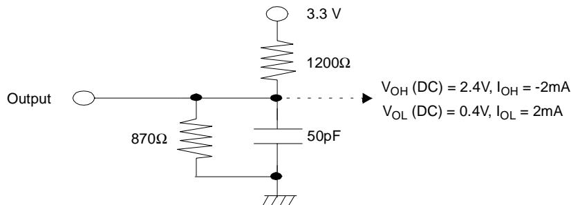
**Output Characteristics** ( $T_A = 0$  to  $+70^\circ\text{C}$ ,  $V_{CC} = 3.3V \pm 0.3V$ )
