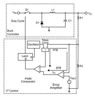
Figure 3. Buck Converter with V<sup>2</sup> Control.
