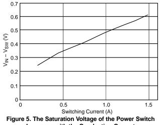
Increases with the Conducting Current
