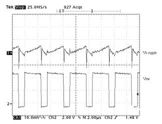
Figure 15. The Output Voltage Ripple Using One 100 µF OS–CON
