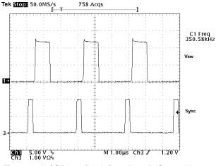
Figure 4. A CS51411 Buck Regulator is Synced by an External 350 kHz Pulse Signal
