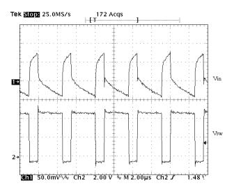
Figure 11. Input Voltage Ripple in a Buck Converter
