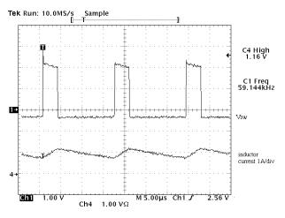
Figure 9. In Short Circuit, the Foldback Current and Foldback Frequency Limit the Switching Current to Protect the IC, Inductor and Catch Diode
