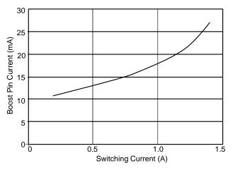
Figure 7. The Boost Pin Current Includes 7.0 mA Predriver Current and Base Current when the Switch is Turned On. The Beta Decline of the Power Switch Further Increases the Base Current at High Switching Current
