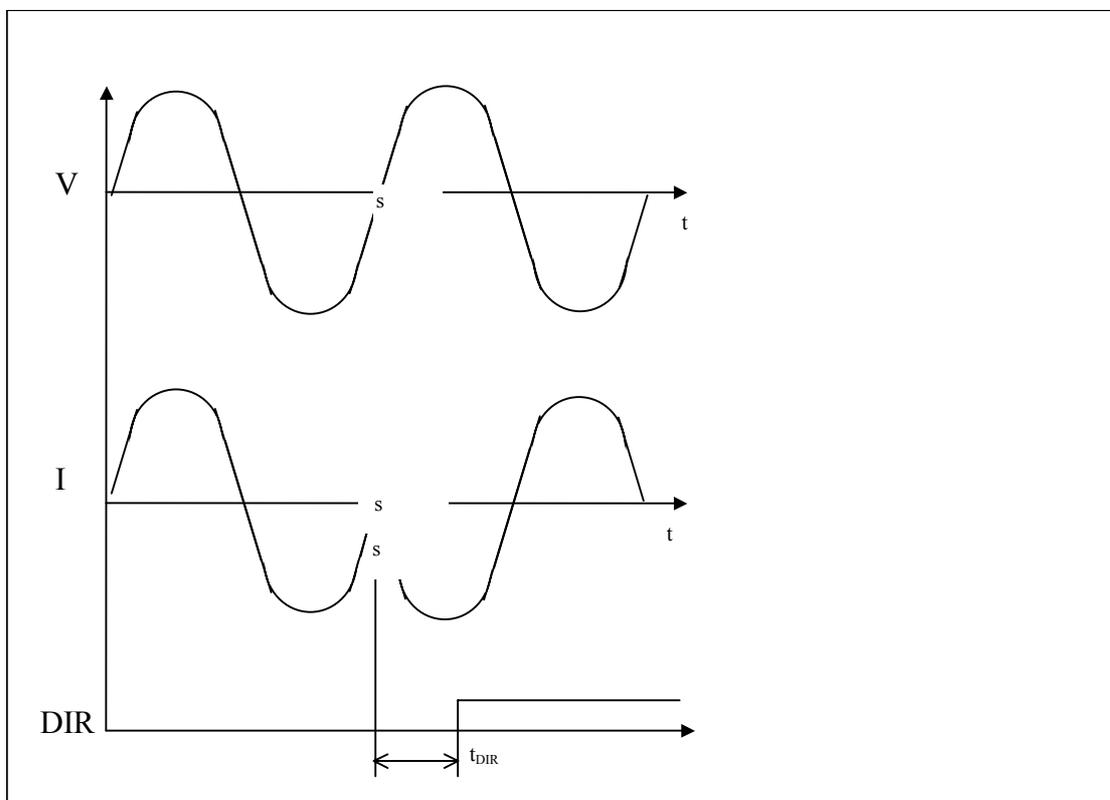
The square wave signal on FMO indicates the polarity of the mains voltage.
