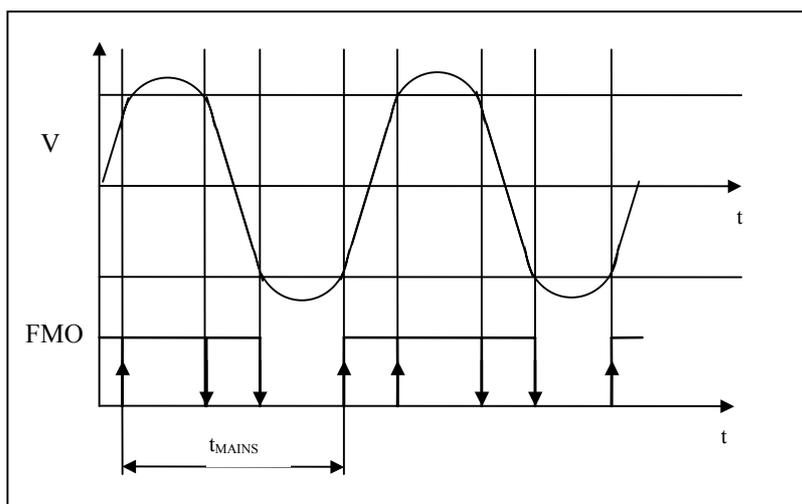
Due to comparator offset, the FMO low to high transition can occur within a range as shown above. The time between successive low to high transitions will be equal to the mains voltage period.
