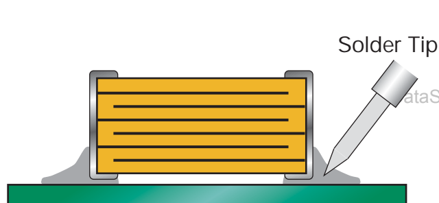
Preferred Method - No Direct Part Contact
