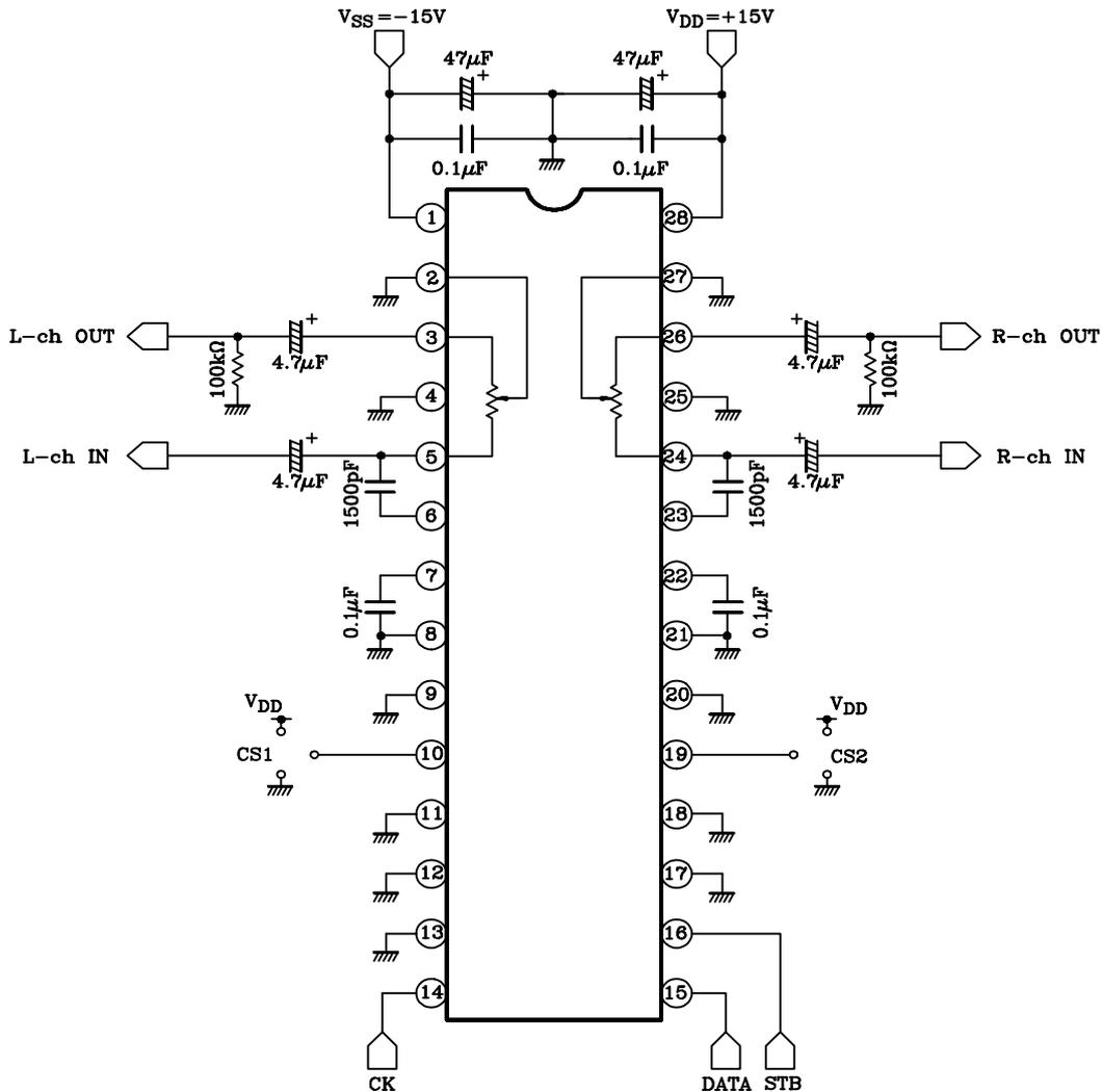
(Note) Since a high-frequency digital signal is input to the CK, DATA and STB pins, corrective measures must be taken to prevent it from getting mixed in the analog circuit to generate noise by, for example, guarding the above signal lines with ground patterns or using shielding wire for these lines.
