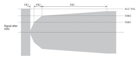
FR value is shown by inclination (FS/s) of the shape of recovery waves. (FS = Full Scale = 0dBFS)
