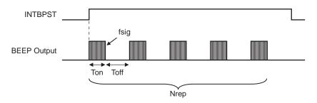
Use the BPHZ register to set the pulse frequency, fsig the BPTON and BPTOFF registers to set the on/off duty, and the BPCNT register to set the repeat count, Nrep. Then set INTBPST =  $0 \rightarrow 1$  to output the BEEP sound. Output stops automatically when the specified number of beeps output.
