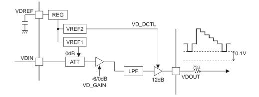
VDIN Sync DC: State of -12.5mV to 162.5mV (At 12.5mV/step, +12dB), -25mV to 325mV (25mV/step, At +6dB) is adjustable to VDOUT Sync DC (100mV).
