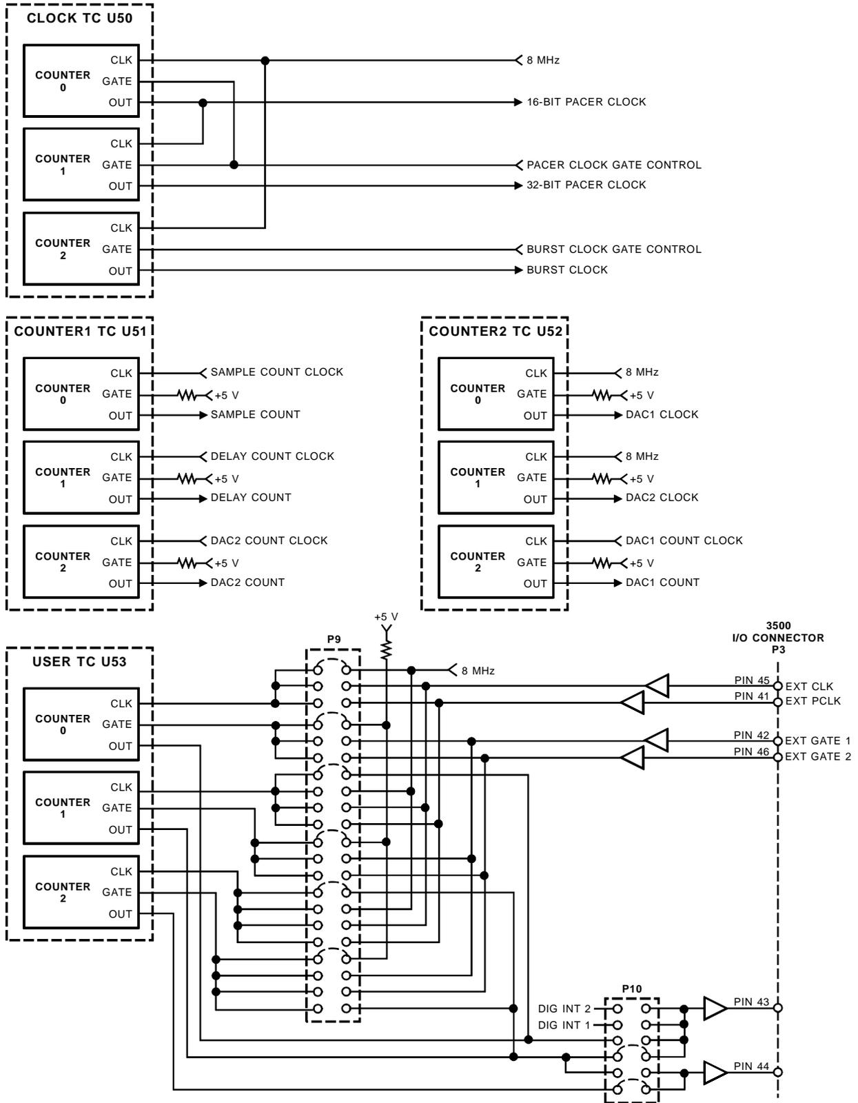
Fig. 9-1 — User TC Circuit Diagram
