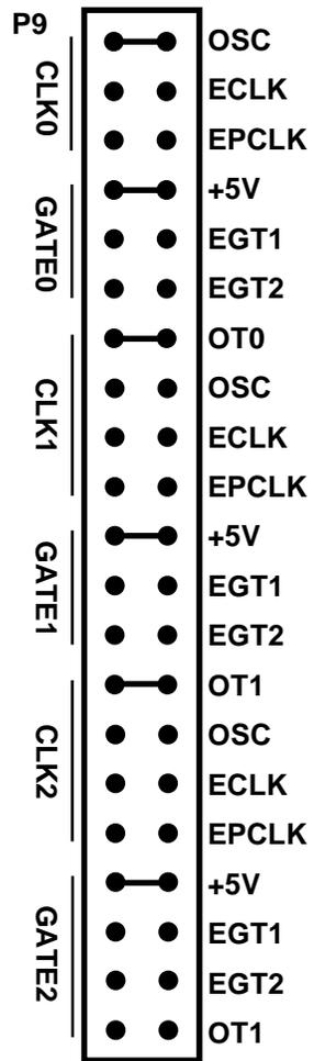
Fig. 1-3 — User TC Clock/Gate Sources Jumpers, P9
