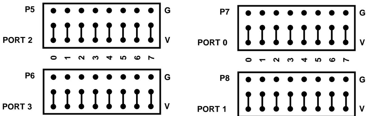
Fig. 1-7 — Ports 0, 1, 2 and 3 Pull-up/Pull-down Resistor Connections
