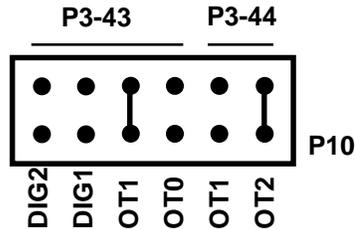
Fig. 1-2 — P3 Signal Select Jumpers, P10
