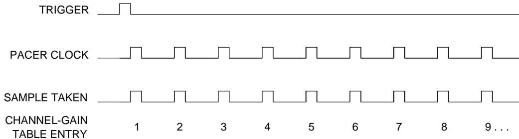
Fig. 5-7 — Timing Diagram, Random Channel Scan
