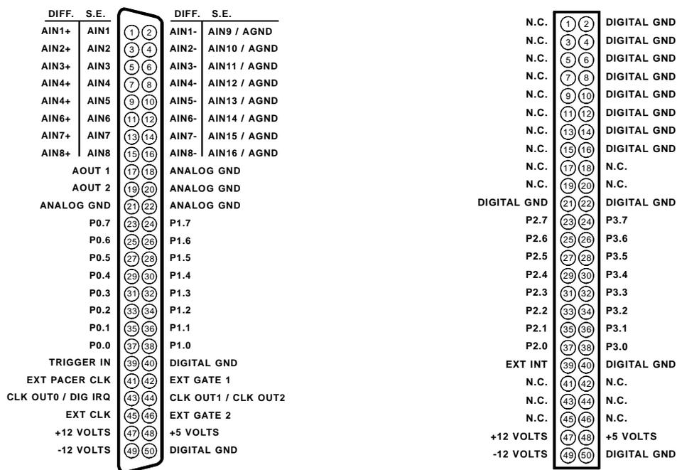
Fig. 2-1 — P3 & P4 I/O Connector Pin Assignments
