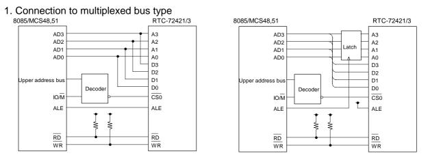
The resistors on the RD and WR lines are not necessary if the CPU does not have a HALT or HOLD state.
