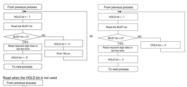
The operation when the HOLD bit is not used involves reading the same digit twice and comparing the read values. This is to avoid the problem of reading unstable data that would occur if the data was read while the RTC was incrementing the count.
