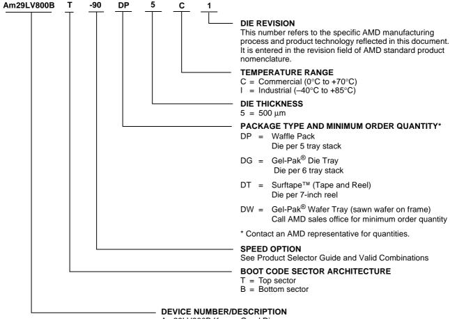
Am29LV800B Known Good Die 8 Megabit (1 M x 8-Bit/512 K x 16-Bit) CMOS Flash Memory—Die Revision 1 3.0 Volt-only Program and Erase
