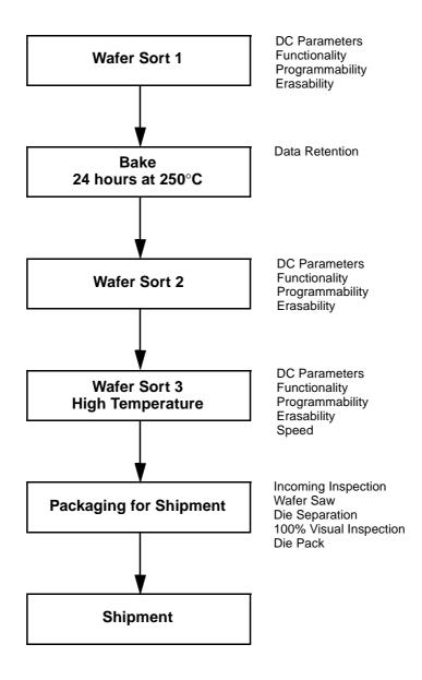
Figure 1. AMD KGD Product Test Flow
