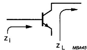
Fig.12 Definition of transistor impedance.
