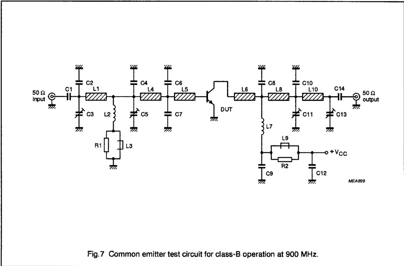
Fig.7 Common emitter test circuit for class-B operation at 900 MHz.
