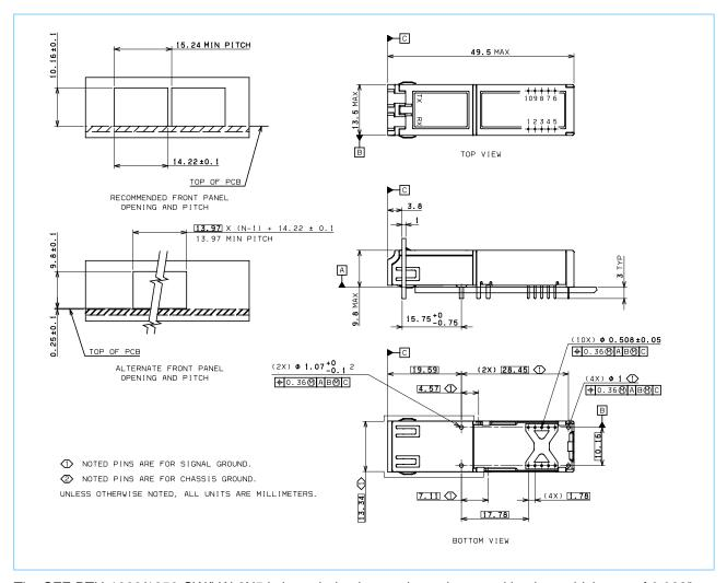
The SFF-PTH-1063/1250-SW/LW-2X5 is intended to be used on a host card having a thickness of 0.062" to 0.100". The host card footprint with essential keepouts and drill holes is shown in Host Card Footprint (2 X 5 Pin Configuration) on page 18.
