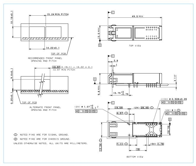
The SFF-PTH-1063/1250-SW/LW-2X6 is intended to be used on a host card having a thickness of 0.062" to 0.100". The host card footprint with essential keepouts and drill holes is shown in Host Card Footprint (2 X 6 Pin Configuration) on page 20.
