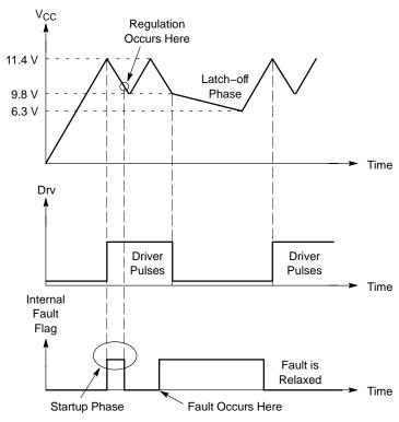
Figure 20. If the fault is relaxed during the  $V_{CC}$  natural fall down sequence, the IC automatically resumes. If the fault persists when  $V_{CC}$  reached UVLO<sub>L</sub>, then the controller cuts everything off until recovery.
