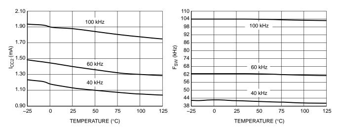
Figure 7.  $I_{CC2}$  vs. Temperature
