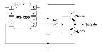
Figure 26. Improving Both Turn-On and Turn-Off Times
