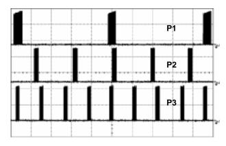
Figure 18. Output pulses at various power levels  $(X = 5 \mu s/div) P1 < P2 < P3$
