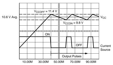
Figure 15. The Charge/Discharge Cycle Over a 10  $\mu F$  V<sub>CC</sub> Capacitor
