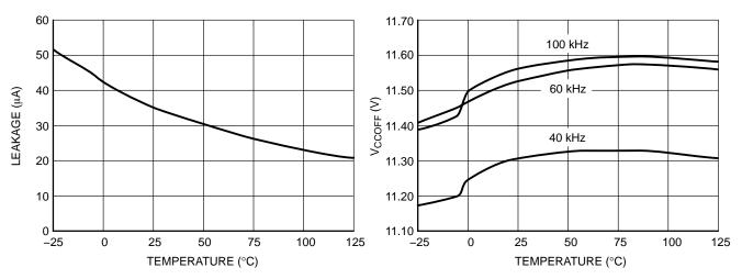
Figure 3. HV Pin Leakage Current vs. Temperature
