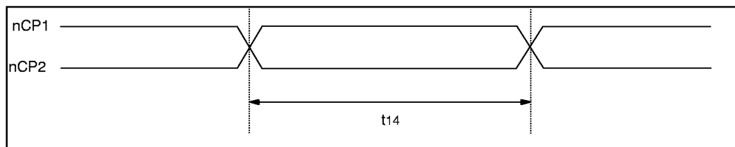
FIGURE 8 – \overline{nCP1} , \overline{nCP2} INPUT TIMING
