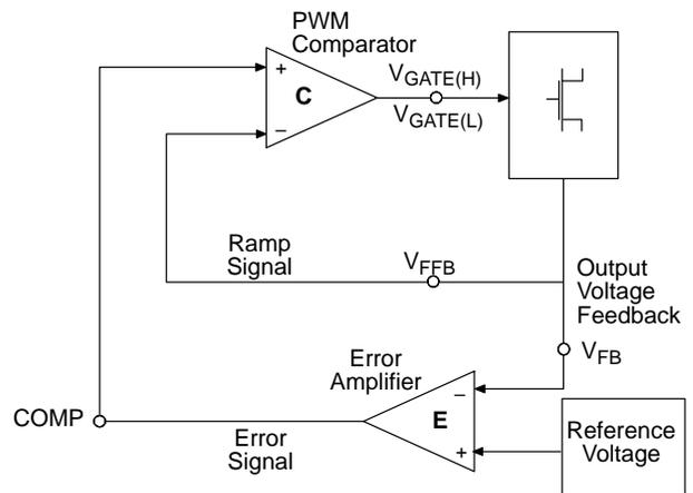
Figure 3. V<sup>2</sup> Control Diagram
