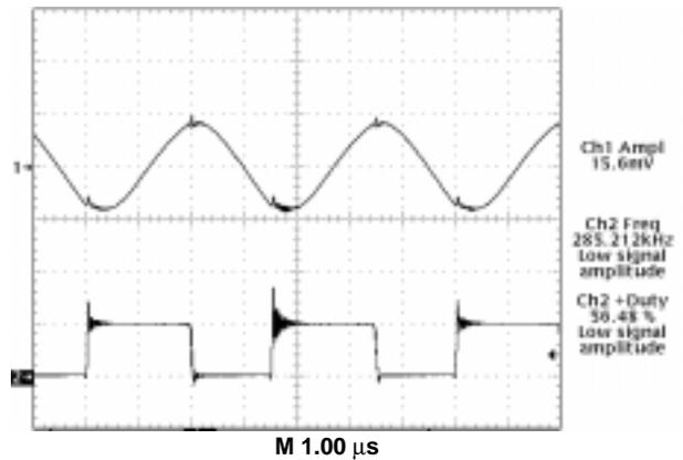
Trace 1— Regulator Output Voltage (10 mV/div.)
