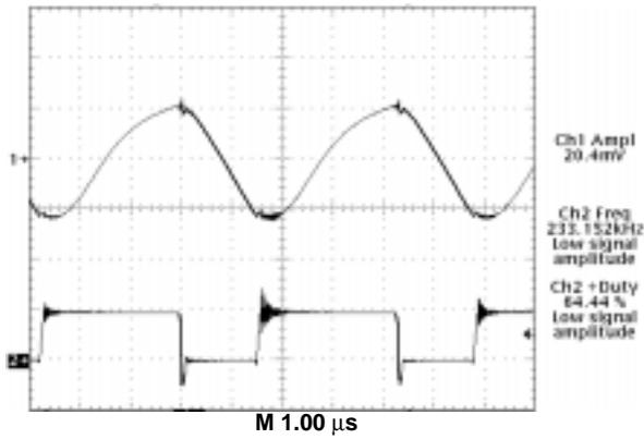
Trace 1— Regulator Output Voltage (10 mV/div.)
