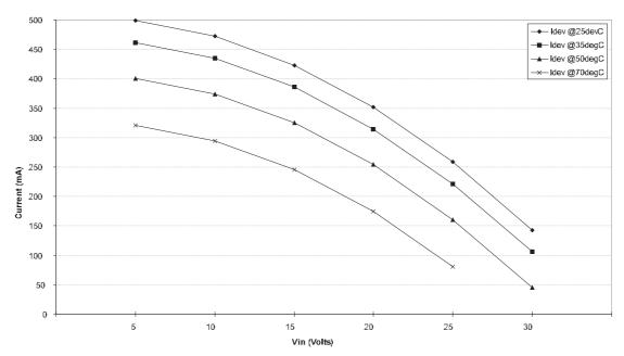
Note- Output channels o to 5 are capable of sinking up to 500mA. Channels 6 and 7 will sink up to 300mA.
