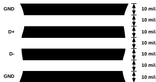
Figure 19. Arrangement of Signal Tracks
