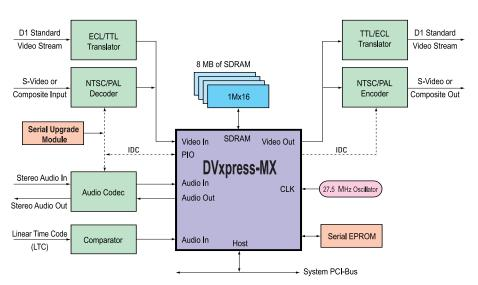
The DVxpress<sup> $\sim$ </sup>-MX Single-Chip Codec Architecture with Glueless Interfaces to PCI, SDRAM, and  $Video\ In/Out$
