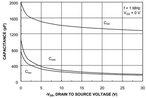
Figure 8. Capacitance Characteristics.
