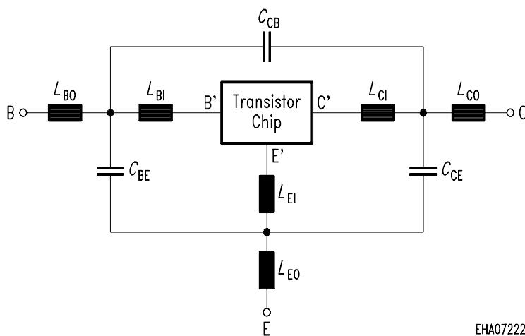
To avoid high complexity of the package equivalent circuit, both emitter leads of TSFP-4 are combined in one electrical connection.  $R_{LxI}$  are series resistors for the inductances  $L_{xI}$  and  $K_{xa-yb}$  are the coupling coefficients between the inductances  $L_{xa}$  and  $L_{yb}$ .
