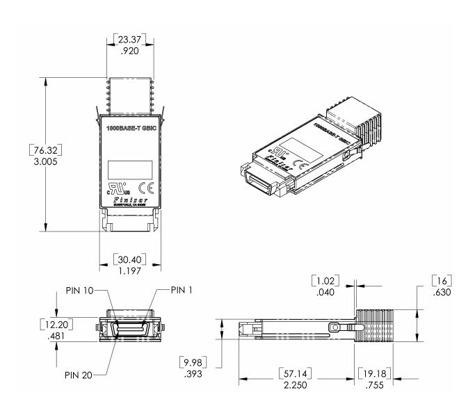
Figure 1. FCL-8520/8521-3 mechanical dimensions
