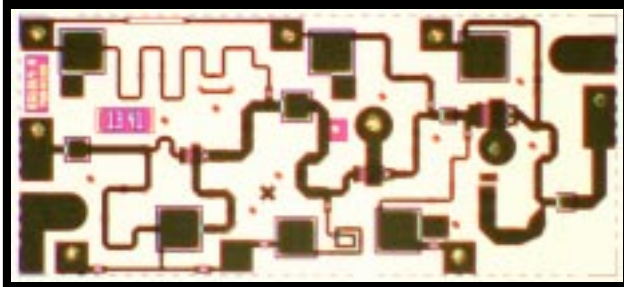
Chip Dimensions 1.984 mm x .923 mm
