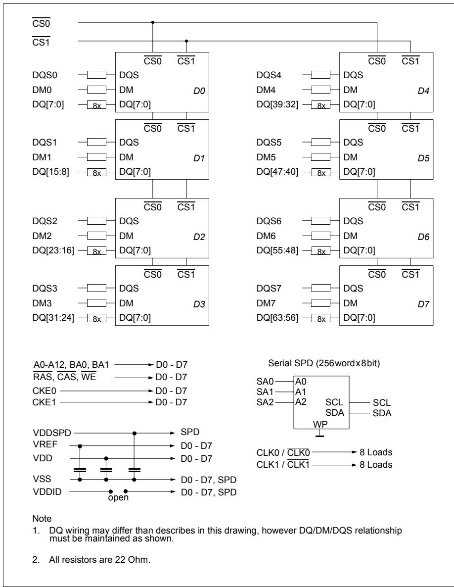
**Block Diagram: Two Banks 128M x 64 DDR-SDRAM SO-DIMM Modules using x8 Organized SDRAMs**
