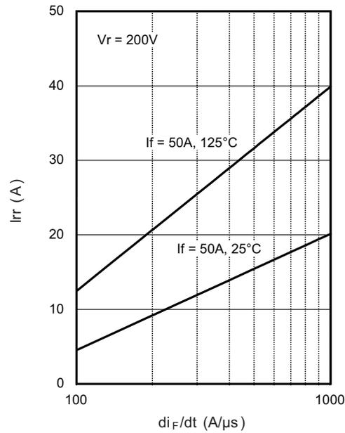
Fig. 9 - Typical Stored Current vs.  $di_F/dt$
