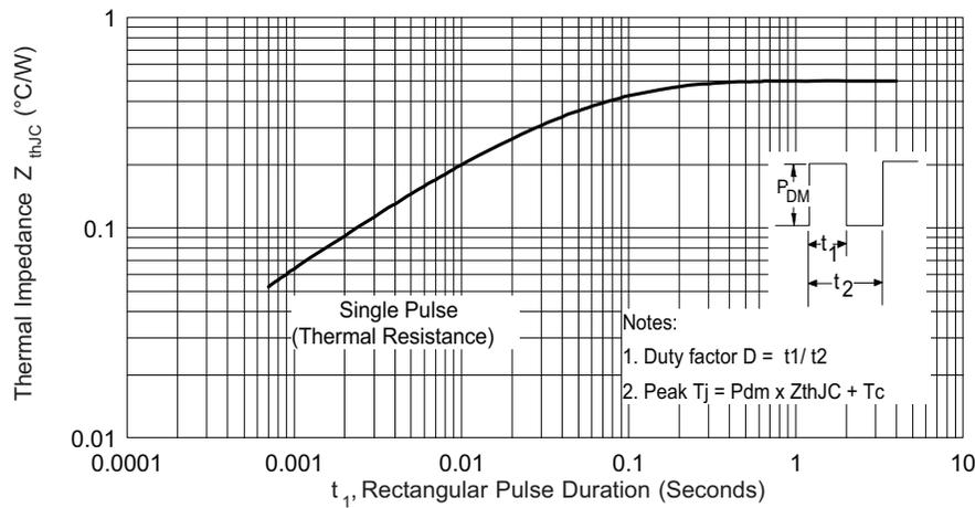
Fig. 3 - Maximum Thermal Impedance  $Z_{thJC}$  Characteristics (Per Diode)
