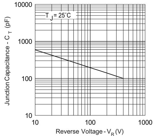
Fig. 2 - Typical Junction Capacitance vs. Reverse Voltage
