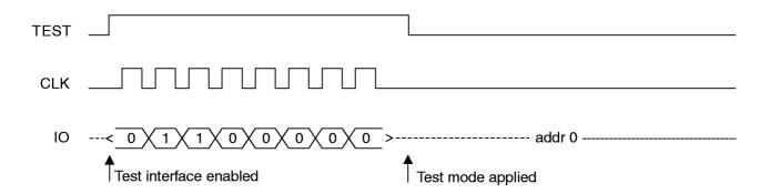
**TEST MODE RESET**: Writing 00H (MSB - > 00000000b < - LSB) to the STR will cause the device to terminate test mode. The STR will contain 00H on power up to indicate normal device operation.
