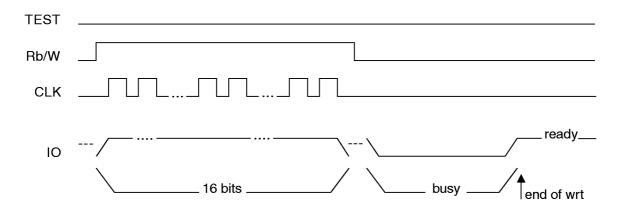
**CORE MARGIN MODE**: This mode is entered with a 07H (00000111b) code. This mode allows cell margins to be tested by placing a test voltage on TEST prior to reading
