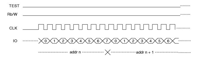
BYTE WRITE: With Rb/W high, shift data starting with the LSB of the byte into the SSR using CLK. When Rb/W falls, the write cycle will be initiated. The ready/busy signal will be present on I/O. A byte write after address preset will
