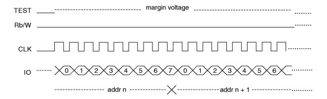
**EVEN PAGE BLOCK MODE**: A code of 04H (00000100b) causes all the even wordlines to be selected. A normal page write should then be executed (see Page Write) to load the data into each even page within the core. This mode, in conjunction with the odd page block mode, allows certain test patterns to be written quickly.
