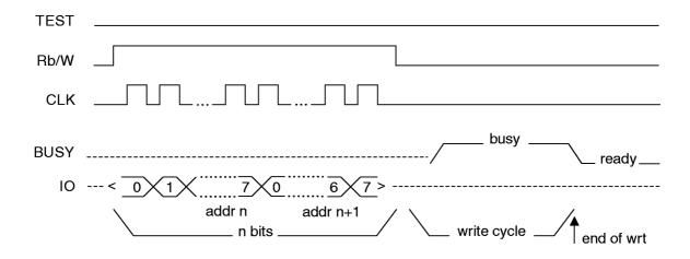
**BLOCK MODE**: Block modes are performed by entering 03H (0000011b) into the STR, which enables all wordlines and bitlines in the core. A block write (zeros) occurs by taking Rb/W high, pulling I/O low, pulsing clock for two bytes
