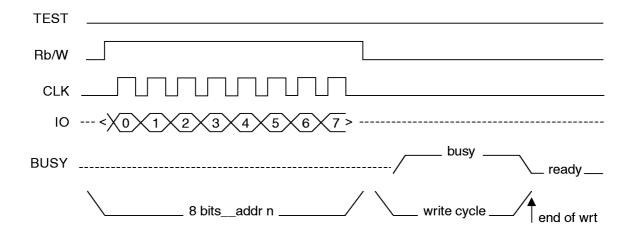
**PAGE WRITE**: This operation allows up to a wordline (512 bytes) to be written at the same time. Perform the same sequence as in the byte write operation "n" times, holding Rb/W high throughout. The address counter will increment as needed to accomplish this. When Rb/W falls, the write cycle will be initiated. The ready/busy signal will be present
