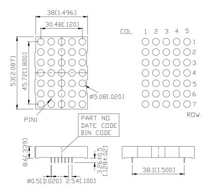
NOTES: 1. All dimensions are in millimeters. Tolerances are  $\pm$  0.25 mm unless otherwise note. 2. Pin tip's shift tolerance is  $\pm$  0.4 mm.
