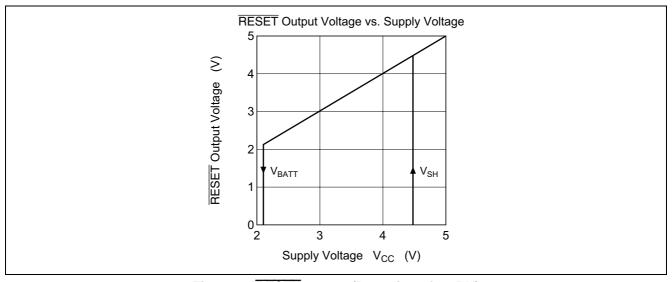
Figure 3 RESET Output (Detection of 2.15 V)
