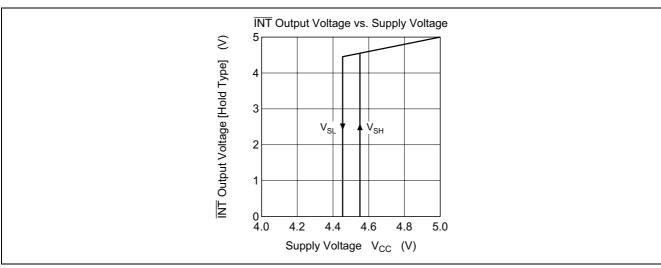
Figure 2 INT Output (Detection of 4.45 V and 4.25 V)
