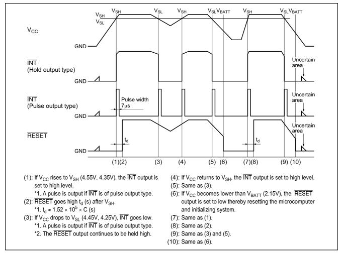
Figure 4 Operating Waveform
