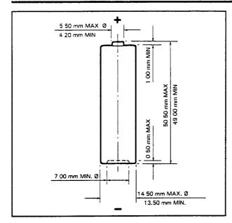
Specification: Nominal Voltage: 1.5 V 2.700 mAh Nominal Capacity: 20.2 h on 10  $\Omega$ Life: to 0.8 V at 20°C Nominal Impedance:  $0.3 \Omega$  at 1 kHz Recomm. Load Range at 20°C: 1 - 15.000 Ω7.4 cm<sup>3</sup> Volume: Average Weight: 22 g I.E.C. Designation: LR6
