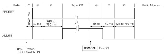
ii) When switched from radio monitor ON in radio mode
