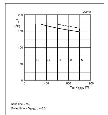
Fig.5 Maximum permissible junction temperature as a function of reverse voltage.
