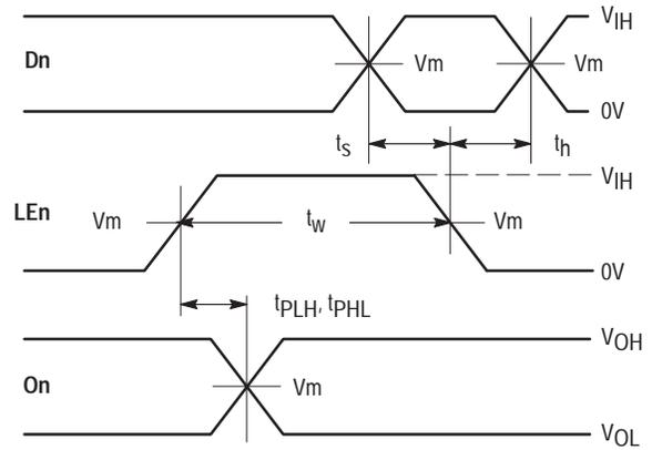
**WAVEFORM 6 - LE to On PROPAGATION DELAYS, LE MINIMUM PULSE WIDTH, Dn to LE SETUP AND HOLD TIMES**
