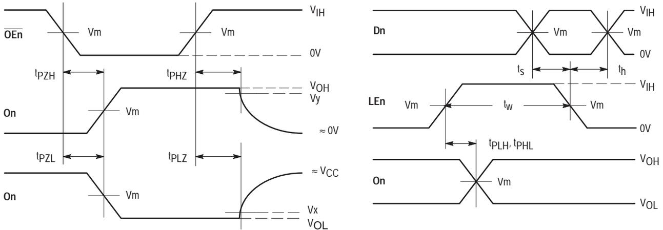
**WAVEFORM 2 - OUTPUT ENABLE AND DISABLE TIMES**
