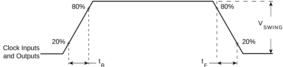
FIGURE 5 - INPUT AND OUTPUT RISE AND FALL TIME
