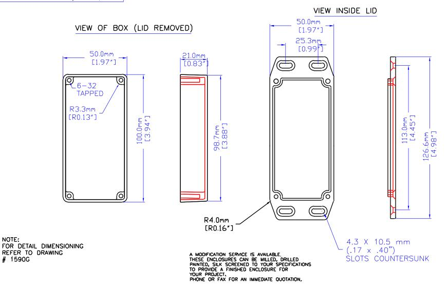
WATERPROOF ENCLOSURE IS AVAILABLE # 1590WGFL, SILICONE SEAL, STAINLESS STEEL SCREWS, THE WATERPROOF ENCLOSURE WILL AFFORD PROTECTION AGAINST LIQUID TO NEMA 4 AND IP65 LEVELS
