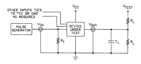
When measuring t<sub>PLZ</sub> and t<sub>PZL</sub>: V<sub>TEST</sub> = 7.0 V.
