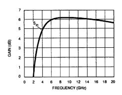
Gain (S $_{21}$ ) vs. Frequency. V $_{\rm DD}$  = 8.5 V,  $\rm t_{\rm DD}$  = 35 mA.
