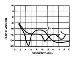
Input Return Loss (S $_{11}$ ) and Output Return Loss (S $_{22}$ ) vs. Frequency.
