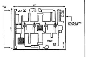
CHIP THICKNESS 5 MILS Au BACKSIDE METALLIZATION
