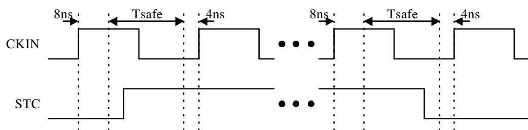
The STC signal is rising-edge triggered, and it should be changed during "Tsafe" region on CKIN .
