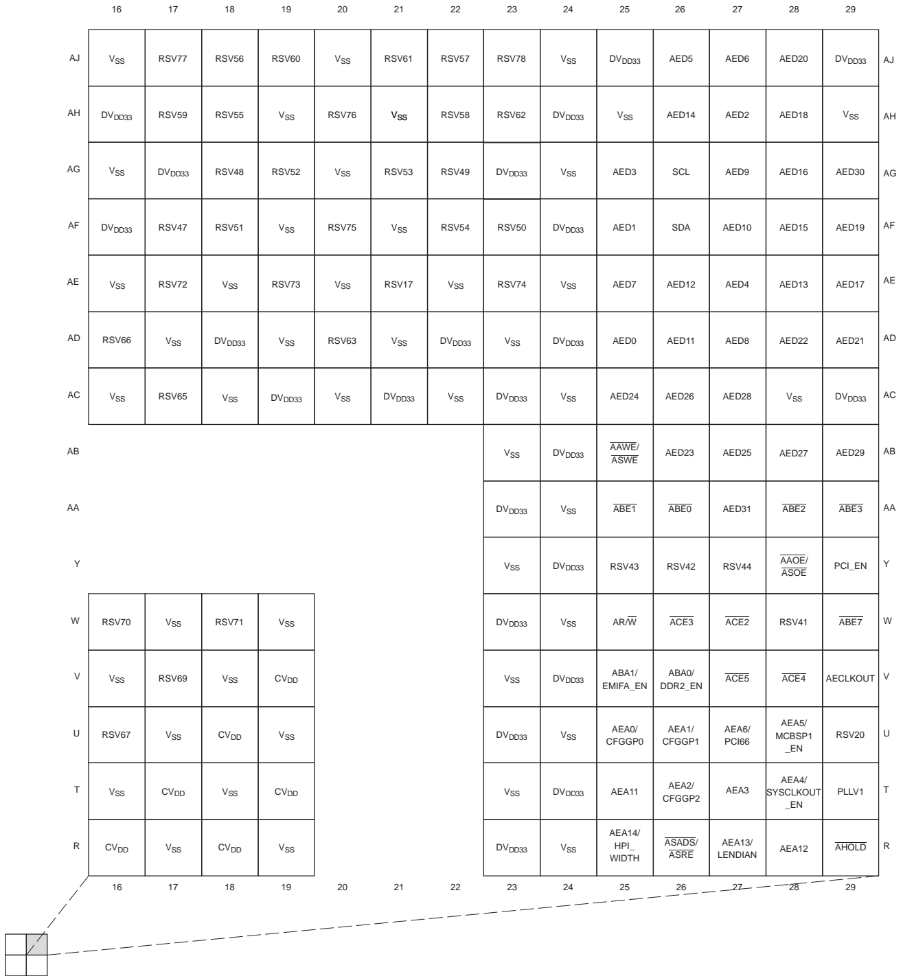
Figure 2-3. C6454 Pin Map (Bottom View) [Quadrant B]
